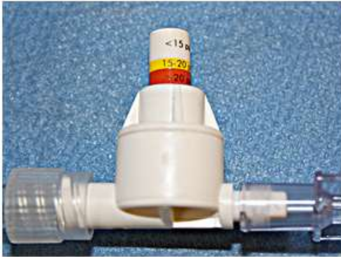
Fig. 1.8 Commercially available single-use, in-line pressure monitor for monitoring injection pressure during peripheral nerve blockade
